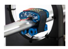
Need to take measurements for a temporary application or in small spaces? Our AT-5000 battery-powered digital telemetry systems are mounted to a shaft using a heavy-duty aramid fiber strap. It measures, digitizes, and transmits data wirelessly off rotating half shafts, drive shafts and rotors to a stationary receiver which converts the digital data to an analog output voltage. These systems are
